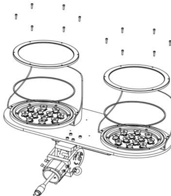
Figure 9 - Diagram of disassembly front cover of Elevated Runway Guard Light
